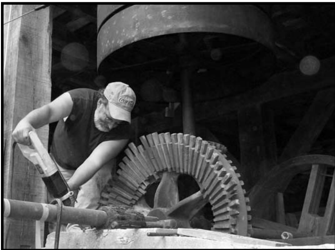
Long-time FMPS volunteer Jimmy High adjusts the shaft that runs from the ring gear to the wheels and belts. Photo by: John Lovett
